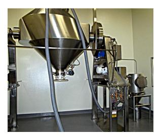
VAC-U-MAX Direct Charge Blender Loading System to a GEMCO Blender. Note the VAC-U-MAX Filter Unit to the right of the blender. System is designed to convey ingredients to the blender from two dump stations.
