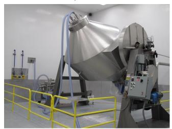
VAC-U-MAX Blender Loading System at a Neutraceutical Company. Conveying Powder to a 150 cubic foot GEMCO Blender.
